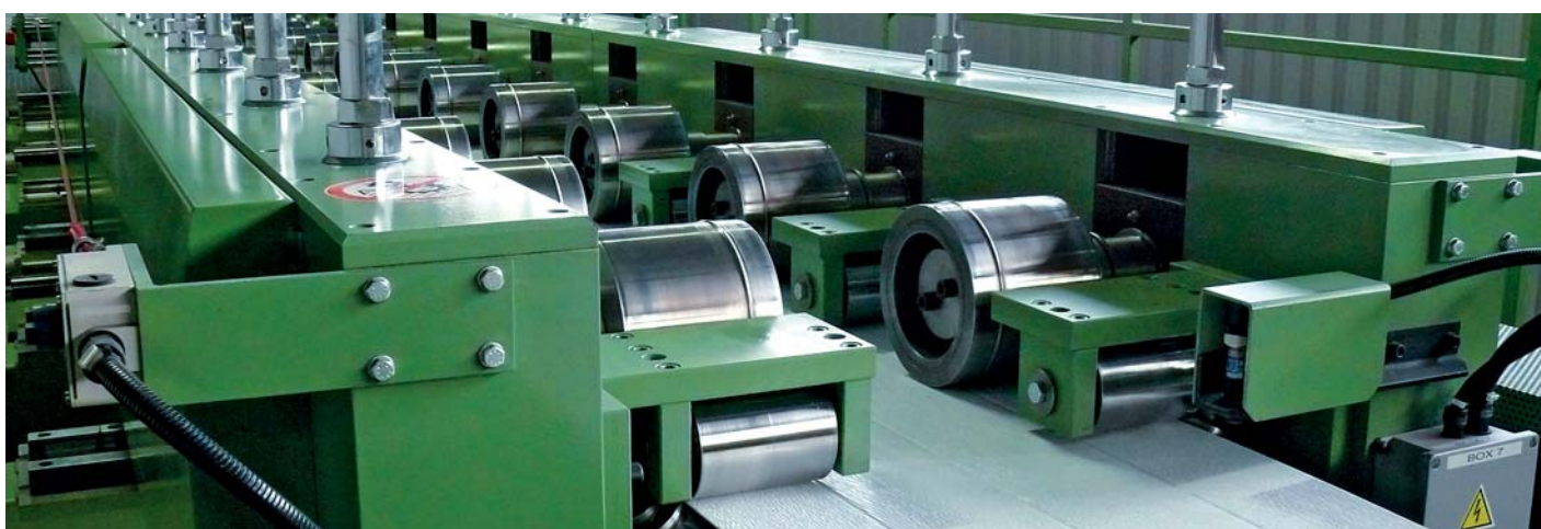
The first stage of panels' production - sheet shaping
