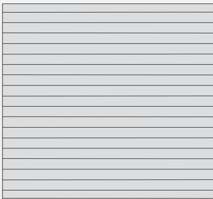
Garage door made of AW 100 profiles
